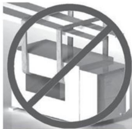
Incorrect Method of Lifting Detector
